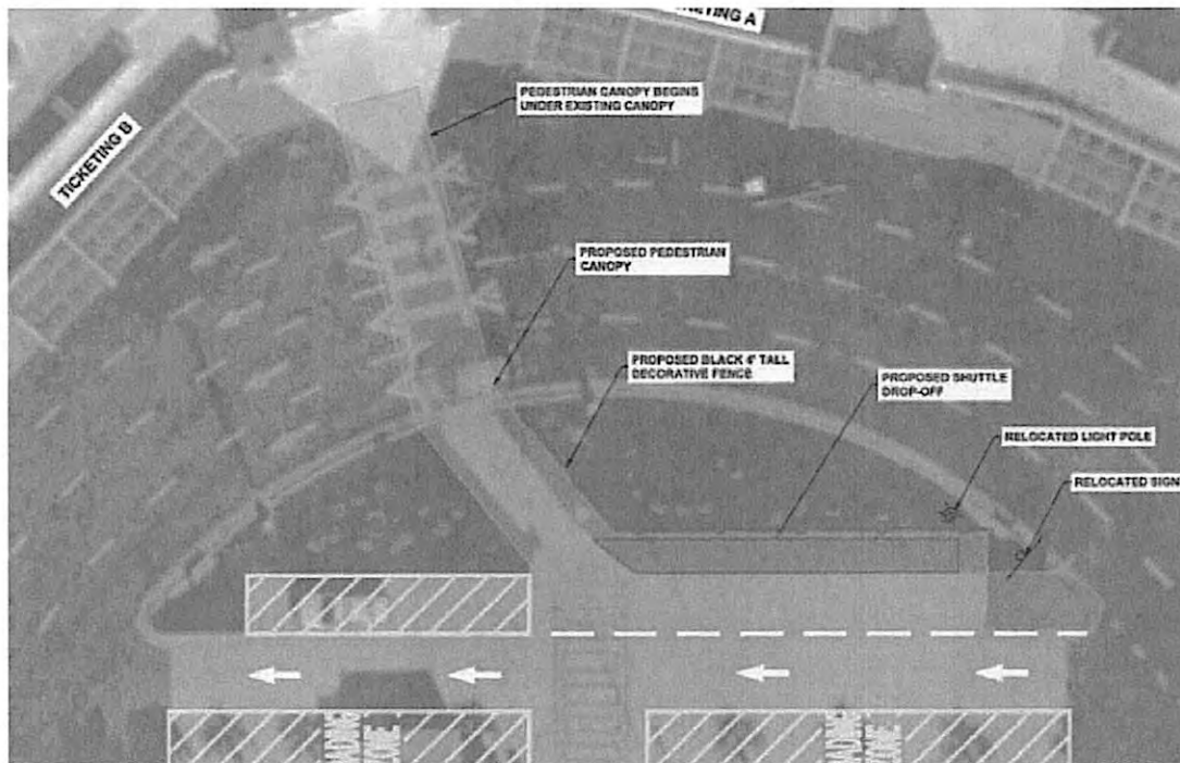
Figure 2: Proposed Modifications to Terminal Shuttle Drop-Off Location
